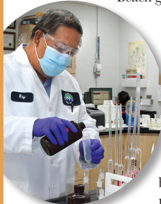
CAWD Laboratory Supervisor Ray DeOcampo prepares samples for coronavirus screening. Wastewater testing can predict COVID-19 spikes by monitoring virus concentrations over time.
