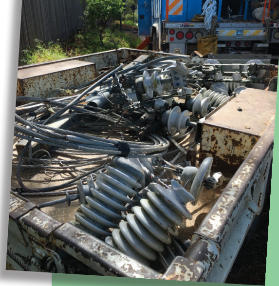
PG&E overhead cable, fuses, and insulators await sorting after their removal from utility poles in Pebble Beach.
