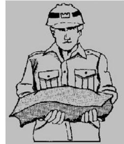
The most commonly use bags are untreated burlap sacks available from feed or hardware stores. Empty bags can be stockpiled for emergency use and will be serviceable for several years if properly stored. Filled bags of earth material will deteriorate quickly.
